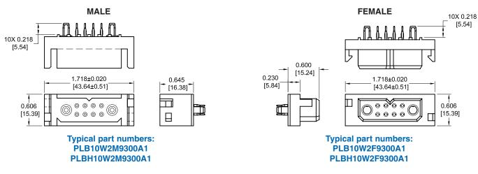
NOTE: Connectors are designed to be mounted to the PCB with screws, see page 63 for mounting screw information. See page 43 for contact hole pattern.
